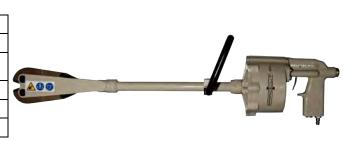
\* Rapidcut 10 Series Cutters are fitted with 1260TM cutter heads, which suits rebar and mesh to 686 Mpa (70kg/mm<sup>2</sup>) yield strength. Typical rebar and mesh sold in Australia is rated at 500Mpa. Please contact your rebar/mesh supplier if in doubt.
